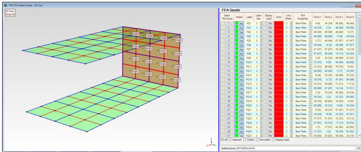
*FEA Plate Model Showing 16 Selected FEA Quads on the Back Plate.*
