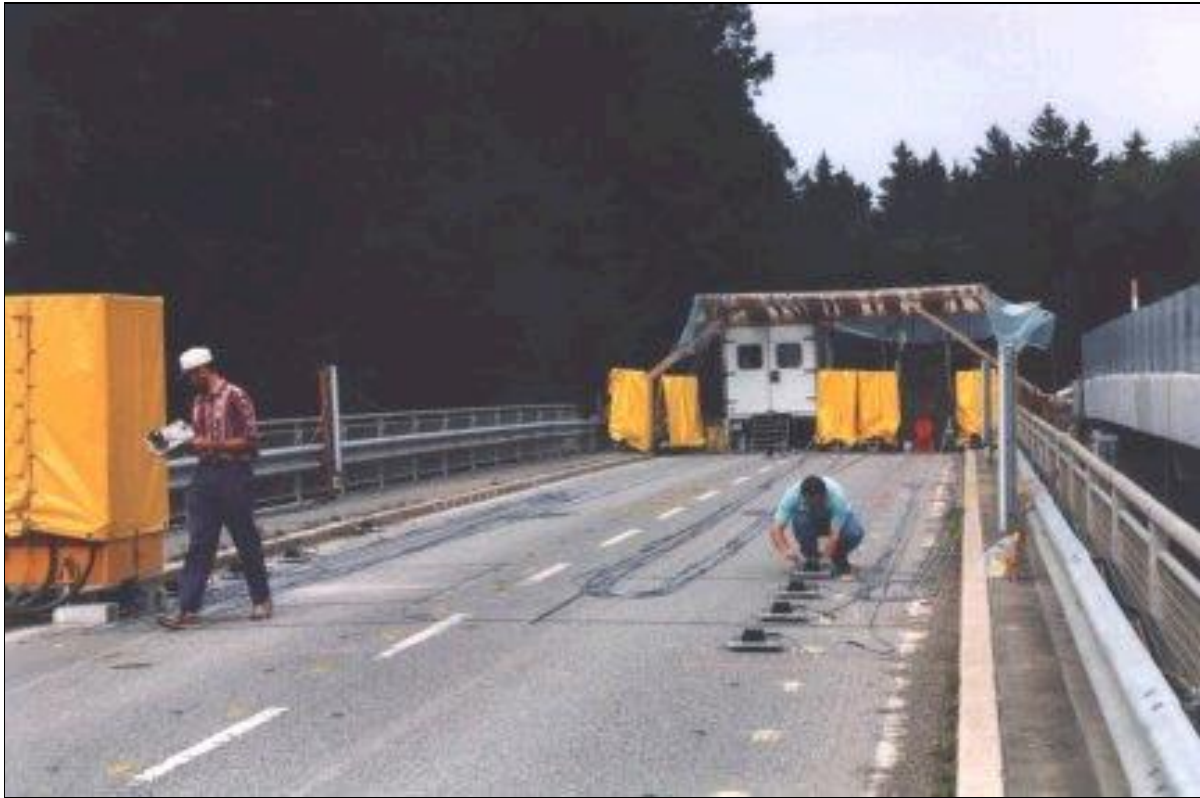
Installing the Accelerometers for one Measurement Set.
