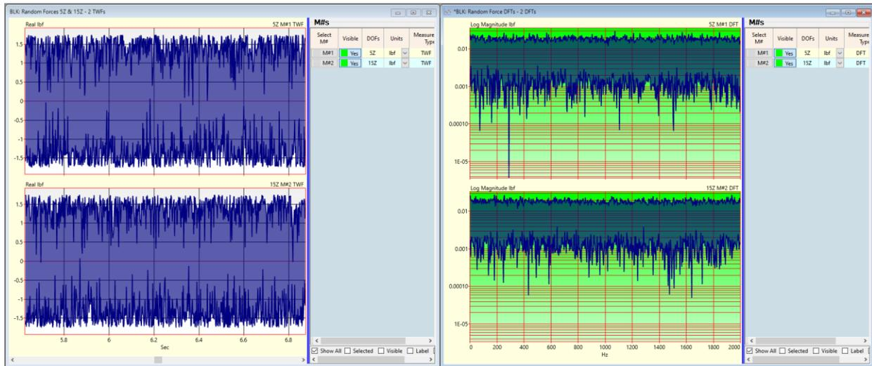
To calculate responses (**Outputs**) at each of the 33 points on the Jim Beam caused by the random excitation forces (**Inputs**), the **EMA** mode shapes are used to synthesize **FRFs** between the **2 Inputs** at **DOFs 5Z & 15Z** and **99 Outputs** at **DOFs 1X, 1Y, 1Z to 33X, 33Y, 33Z**.
