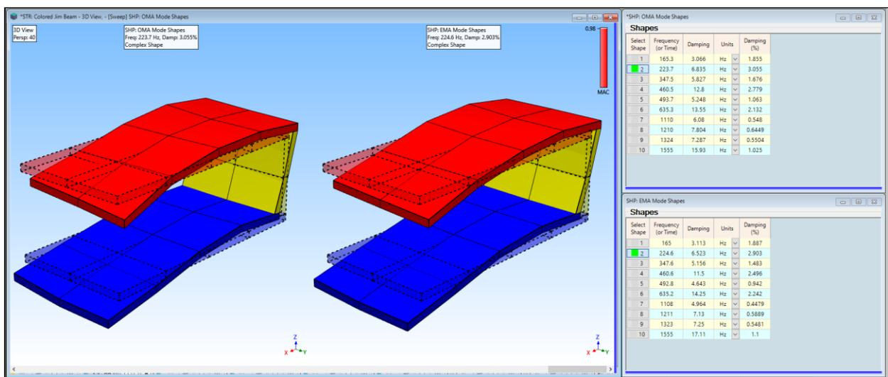
OMA Mode Shape on the Left and EMA Mode Shape with Maximum MAC on the Right.
