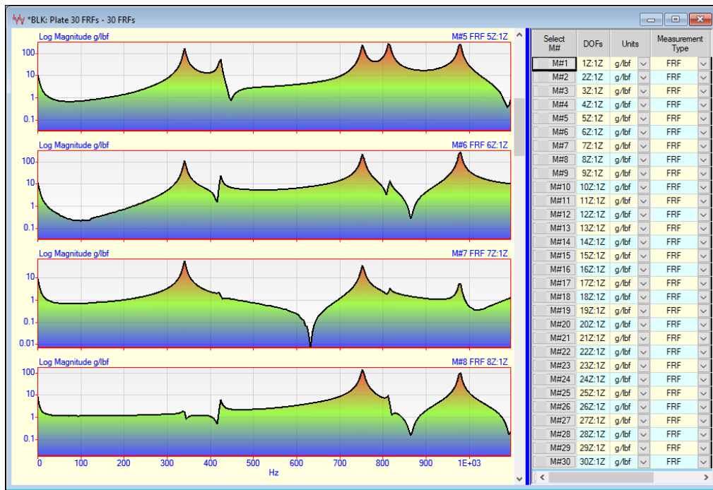
Experimental FRFs from a Roving Impact Test of the Aluminum Plate.
