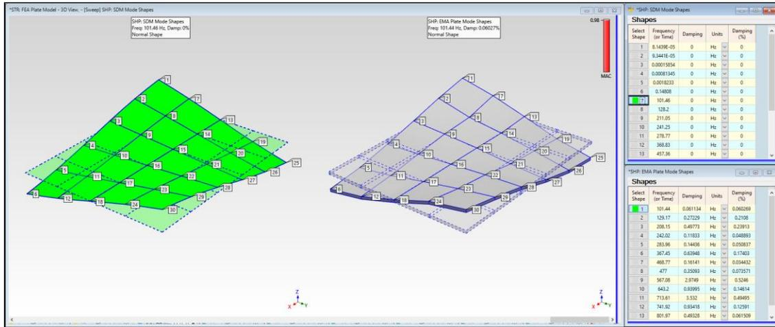
Animation of an **SDM** Mode Shape Side-by-Side with the Closest Matching **EMA** Mode Shape.
