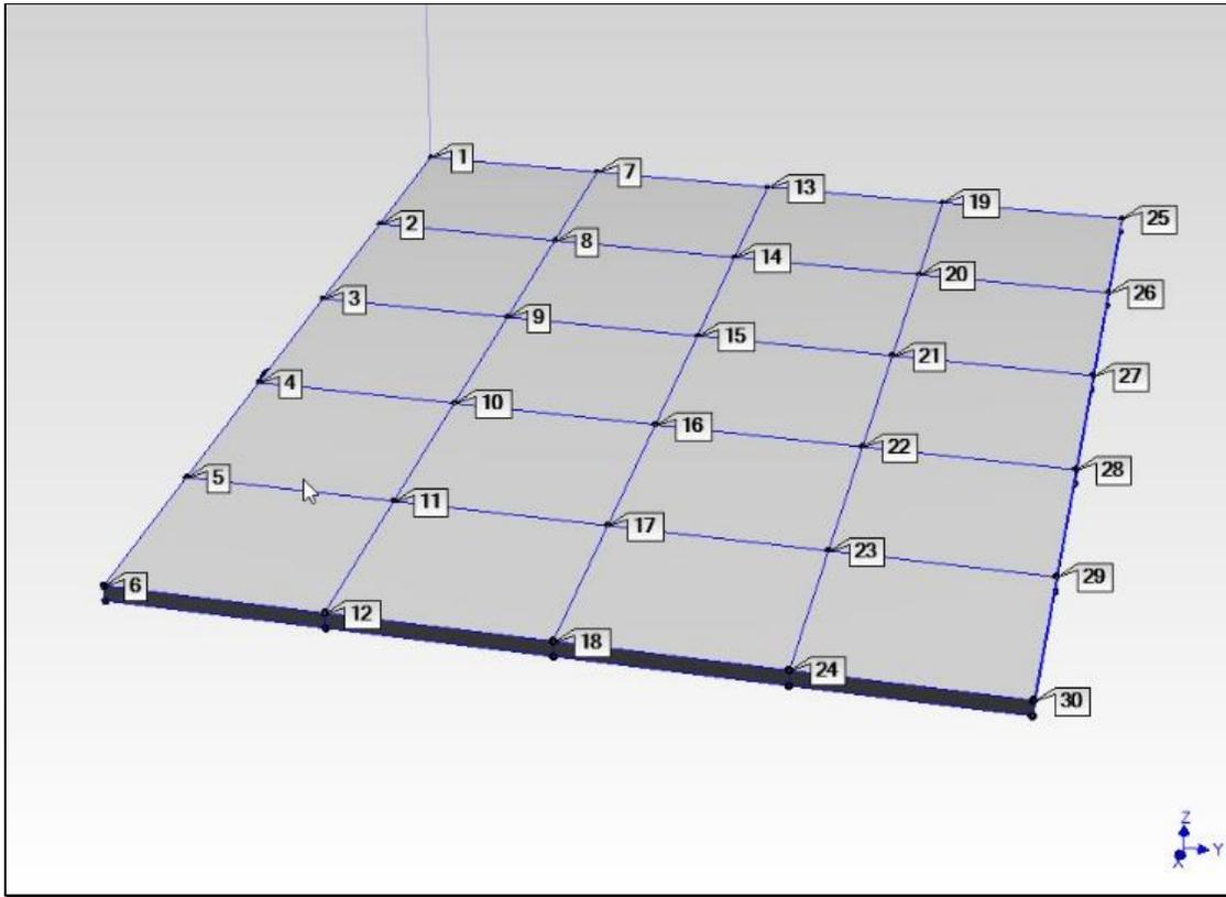
Impact Test Points for Roving Impact Modal Test.
