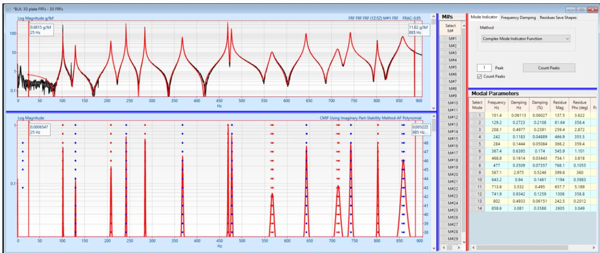
Curve Fit of an Experimental FRF.
