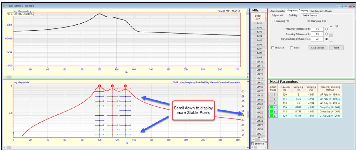
Stability Diagram Showing **Stable Pole Groups** from **Complex Exponential** Curve Fitter
