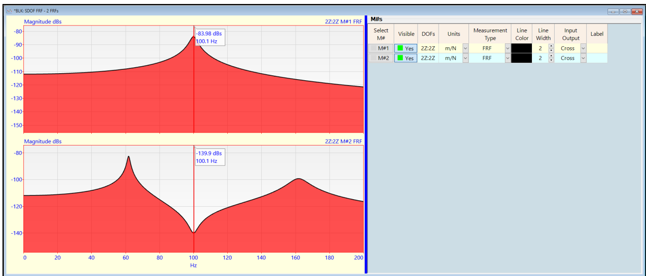
Driving Point FRFs Before & After the Tuned Absorber is Attached to the SDOF Model .
